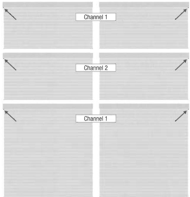
As a general rule, the infrared eyes on adjacent shadings should be positioned as far apart as possible for independent operation of each shading, using a single channel. The minimum separation for independent single-channel operation is 48". Two-channel operation may be required with stacked configurations to ensure independent operation of each shading.
