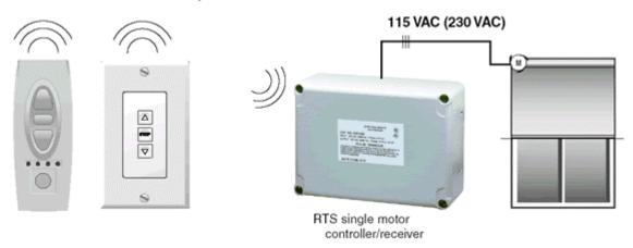
With the Radio Remote Control System (RTS<sup>TM</sup>) you can remote control any standard motor within a 65-foot range that is wired to an RTS single motor controller/receiver. RTS offers all the same ease and convenience of the RTS<sup>TM</sup> System without the need for an intelligent motor.
